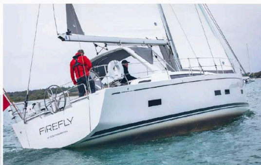
The cockpit arch gives the mainsheet a good mechanical advantage while keeping it clear of crew
