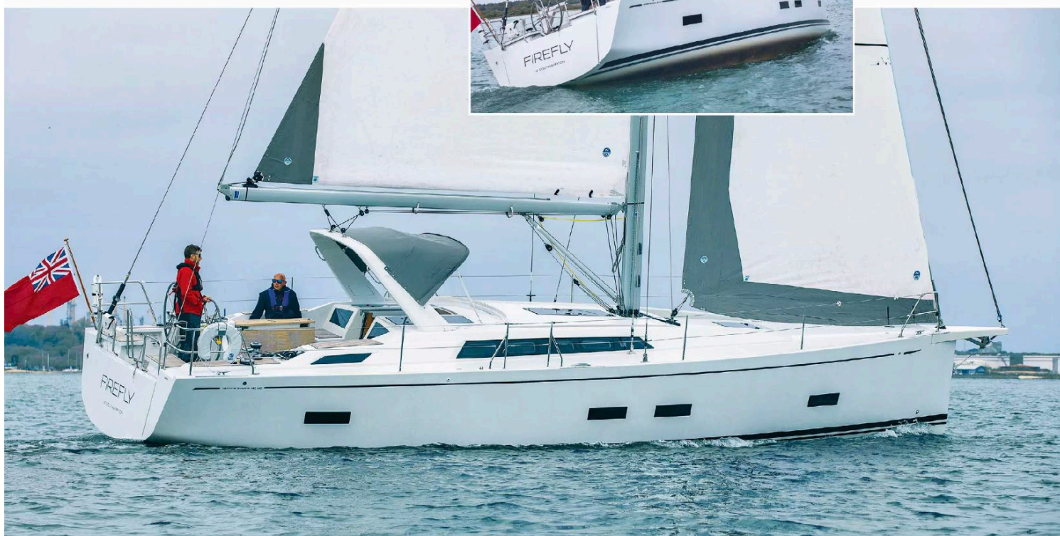
The cockpit arch gives the mainsheet a good mechanical advantage while keeping it clear of crew
