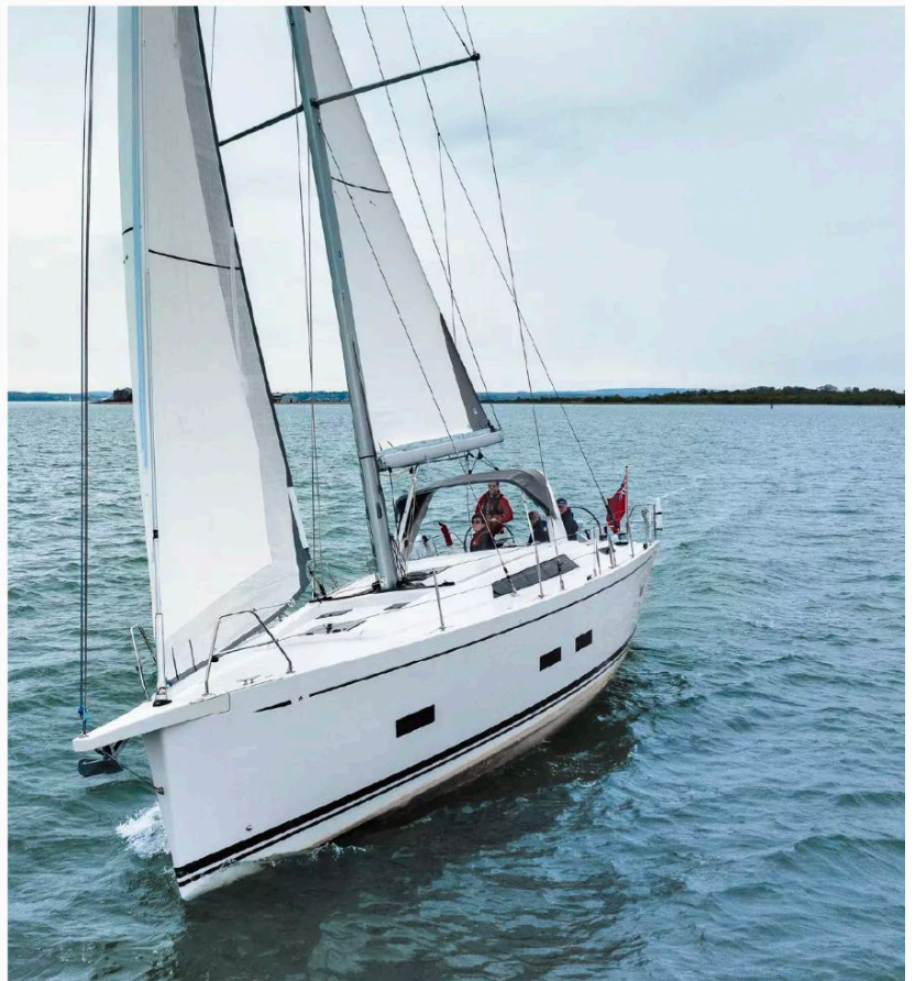
A narrow waterline forwards and fair lines aft help the boat point well and get moving quickly
